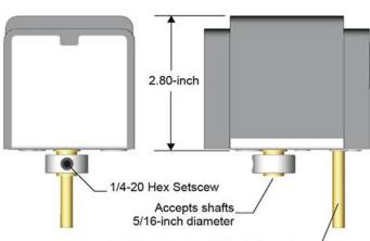
Anti-Rotation Pin, .25-inch diameter \_\_\_\_
